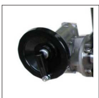
Handwheel drive to turn the tank
